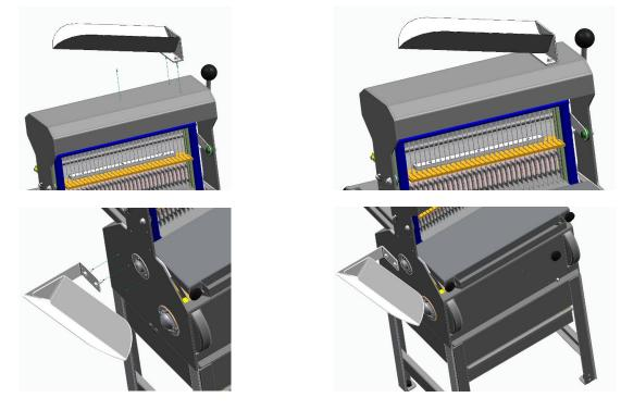
Installing the Front Bagging Scoop (as applicable)
